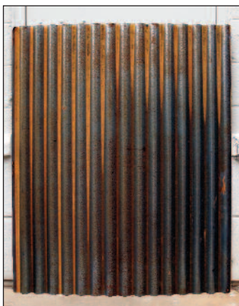
Right: Cor-ten corrugated steel panel after three weeks of exposure outside
